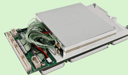
10.1×5.4×1.9cm/127g 2Watts×2/4Watts×2 (7Z100) (Air to G. 20~100/100~150KM)
