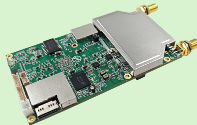
11.5×5.4×1.3cm/56g 4Watts×2/5Watts×2 (Air to G. 100~150/100~200KM)
