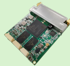
5.8×4.8×1.0cm/27g 0.5Watts×2/1Watts×2 (Air to G. 10~30/20~50KM)
